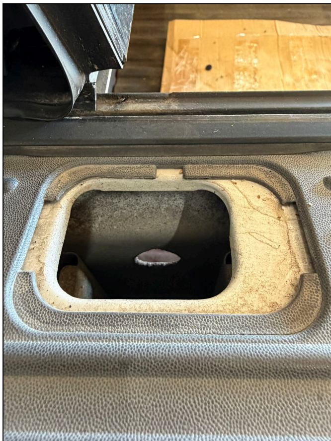
4. Cover Removed – Showing Top Mount Hole
