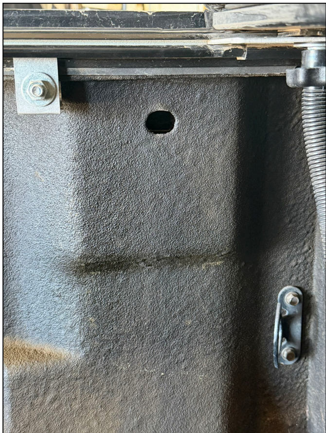
1. Driver Side Install Location – Note Tonneau Clamp
